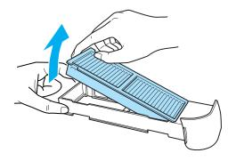
Install the new air filter into the air filter cover.
