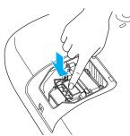
Tighten the lamp fixing screw.
