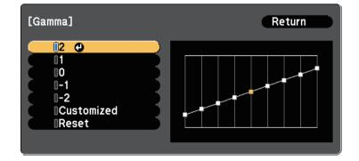
When you select a smaller value, you can reduce the overall brightness of the image to make the image sharper. When you select a larger value,
