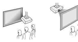
Make sure you select the correct **Projection** option in the projector's **Extended** menu according to the installation method being used.
