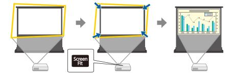
The projector's sensor can detect the screen size and shape in these conditions:
